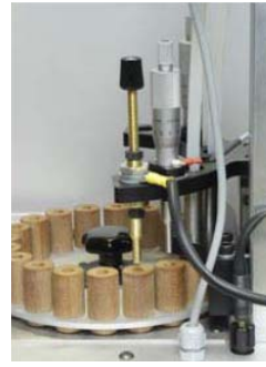
The EVO System can be equipped to stress relieve and load test springs in-line prior to delivery to an assembly station
