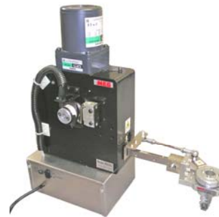
Cam Actuated Air Valve for Gripper Control
