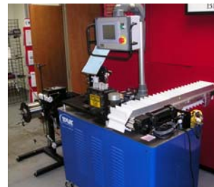
#2 Servo Linear Feed System with Touch Screen Interface, #3 Quill-On-Quill Cutter Head, Batching Conveyor and High Speed Payoff
