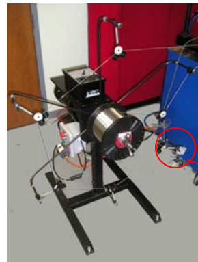
High Speed Fine Wire Payoff with Lanyard Speed Potentiometer
