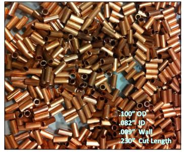
Shear Cut Copper Tube Ferrules
