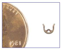
Industry – Electronic / Switch Material – NiCu 101 Rolled Wire
