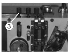
Adjusting screw for feed roll pressure
