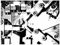
Correctly adjusted spring. The spring is centered according to the cutting line
