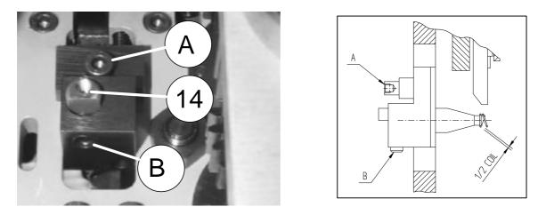
NOTE: When winding, the spring is not to come in contact with the mandrel!
