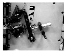
Micrometer for spring diameter
