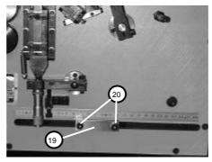
The machine is designed for a maximum wire length of 1200 mm. In order to obtain the best possible precision when making a spring of shorter wire length, the machine is normally delivered with an gearing suited for spring in question. The unit can be delivered for a maximum wire length of 100, 200, 300, 400, 600, 900 and 1200 mm. To replace the gear, Please contact your sales representative.
