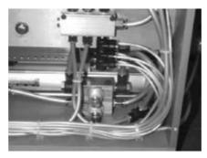
Valves for adjusting speed Upper valve for return stoke
