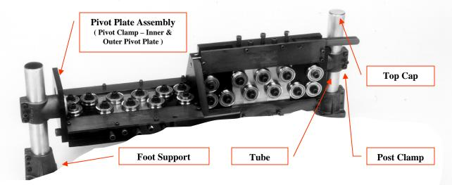
The TAK series #04 & #05 come in two configurations. Selection of the QR ( Quick Release ) version requires a slightly different approach to mounting other than a simple angles bracket with holes. The three methods are listed below:
