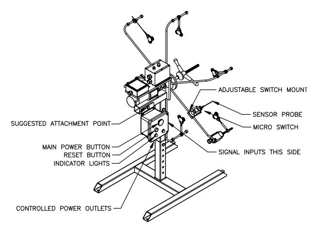
This system is designed to provide an automatic shutdown of any equipment attached to the controlled outlets. This system also requires a "manual reset" to restore power to any equipment attached to the controlled outlets.
